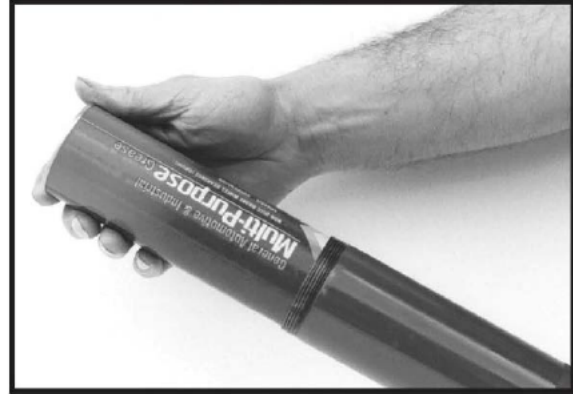
Installing Grease Cartridge
