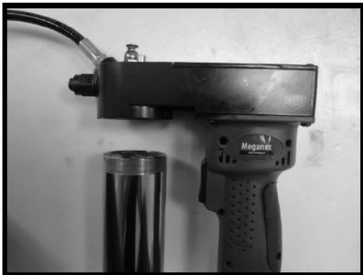
Rotate grease container counter clockwise to remove. Turn clockwise to tighten.
