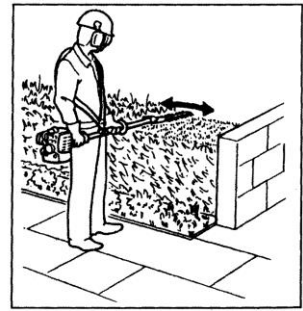
Horizontal cutting: Cutting without standing directly in front of the hedge, e.g. reaching over a flowerbed.
